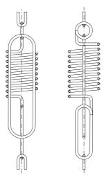
It is hooked onto the suspension chain of the displacer in place of 7 chain links (105 mm). This spring is specially matched to the resonance frequency of the displacer and is made of stainless steel (1.4310, operating temperature up to  $250\,^{\circ}\text{C}$ ).
