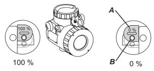
After shifting the key protection cap  $\boldsymbol{A}$ , insert screw driver or pin ( $\emptyset$  < 3 mm) into hole  $\boldsymbol{B}$  and press down to the second pressure point.
