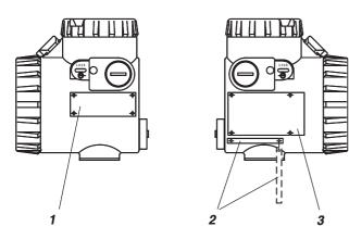
The transmitter is identified with several labels. The transmitter nameplate 1 shows the Model Code of transmitter, which clearly describes the device. The certificate data and the serial No. are shown on the amplifier nameplate 3. The optional TAG No. label 2 with the Tag No. is located underneath.
