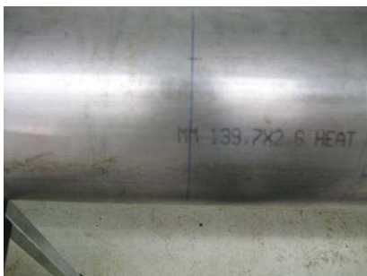
Picture 28 Pipe with first mounting line for first transducer
