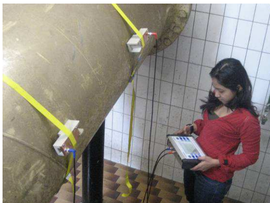
Picture 18 Example of the V-mode mount with fabric-reinforced tensioning tapes for large pipe diameters
