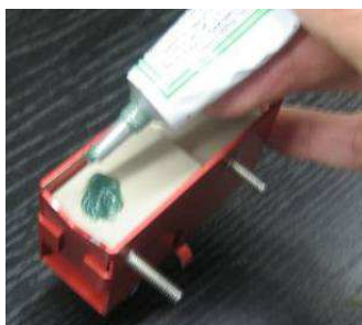
Picture 23 Proper application of the acoustic gel on the sensing face of the ultrasonic transducer
