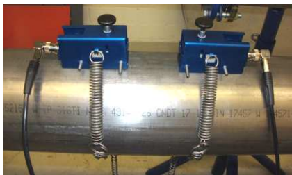
Picture 16 Example of the V- or W-mode without spacer bar
