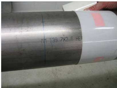
Picture 30 Set up the template to mark the mounting position of the second transducer
