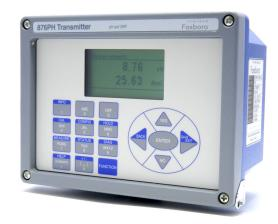
The Foxboro<sup>®</sup> brand Model 876PH is a 2-wire loop powered intelligent transmitter that, when used with appropriate electrochemical sensors, provides measurement, local display, and transmission of pH, ORP (Oxidation-Reduction Potential), or ISE (Ion Selective Electrode) concentration. The transmitter outputs a HART digital signal and a 4 to 20 mA analog output.
