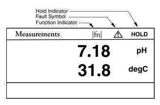
Figure 3. Typical Dual Measurement Display
