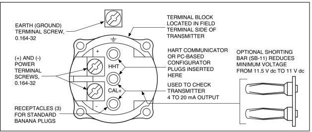
Figure 23. Field Terminal Block
