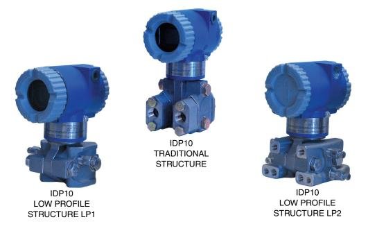
The Foxboro<sup>®</sup> brand I/A Series<sup>®</sup> Model IDP10 is an Intelligent, two-wire d/p Cell<sup>®</sup> transmitter that provides precise, reliable, measurement of differential pressure, and transmits a 4 to 20 mA output signal with a superimposed HART<sup>®</sup> digital signal for remote configuration and monitoring.
