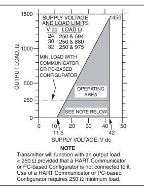
Figure 19. 4 to 20 mA Output, Supply Voltage vs. Output Load
