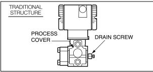
Figure 4. Vertical Mounting - Cavity Draining
