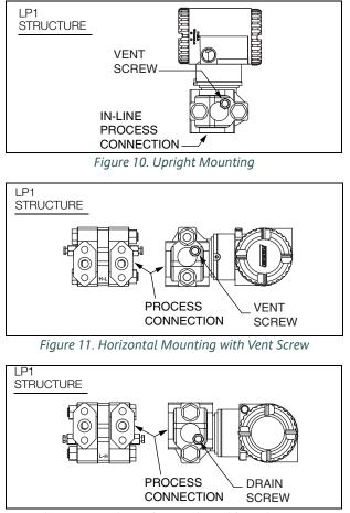
Figure 12. Horizontal Mounting with Drain Screw
