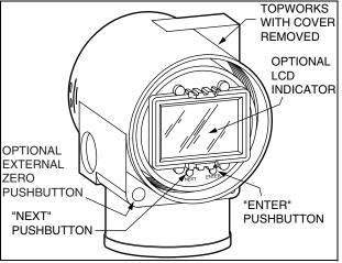
Figure 22. LCD Indicator with On-Board Pushbuttons
