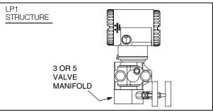
Figure 8. LP1 Shown Directly Mounted to Manifold
