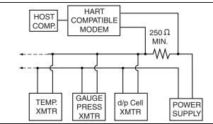
Figure 21. Typical Multidrop Block Diagram
