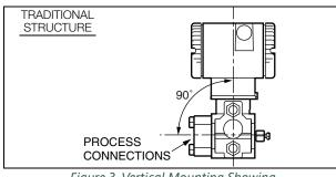
Figure 3. Vertical Mounting Showing Process Connections at 90 degrees
