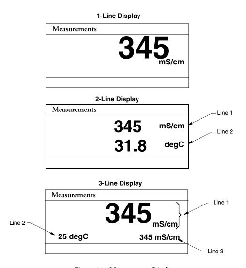
Figure 21. Measurement Display
