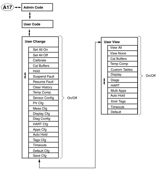
Figure C-17. Passcode Access Structure
