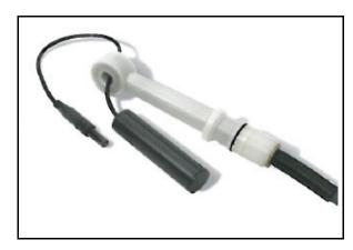
EP485 Calibration Plug with 871FT Sensor
