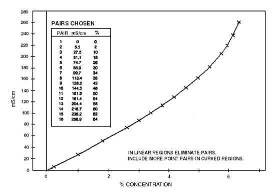
Figure 19. Configured Conductivity vs. Concentration Data
