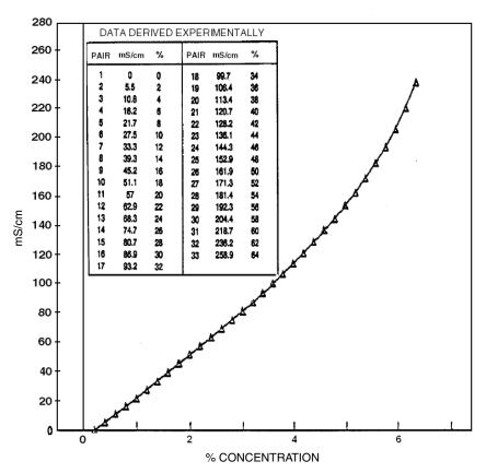
Figure 18. Reference Conductivity vs. Concentration Data
