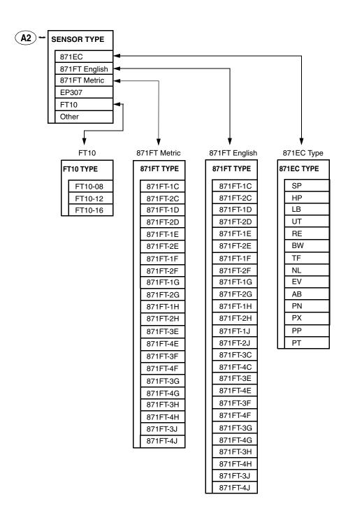
Figure C-2. Sensor Type Configuration Structure
