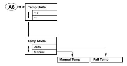
Figure C-6. Temperature Configuration Structure
