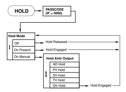
Figure 14. Hold Mode Menu Structure Diagram
