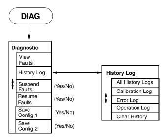
Figure 23. Diagnostic Mode Structure
