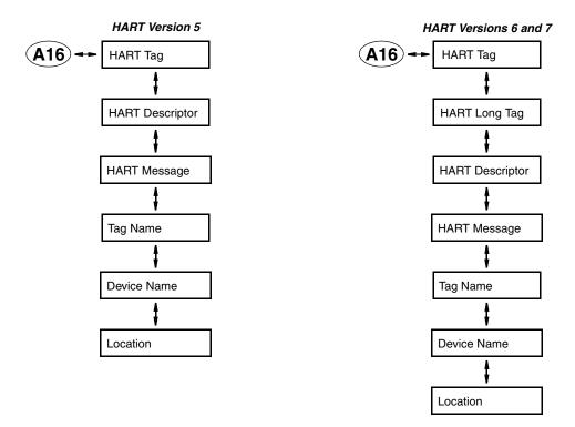
Figure C-16. Transmitter Tags Structure
