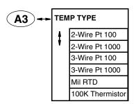
Figure C-3. Temperature Type Configuration Structure
