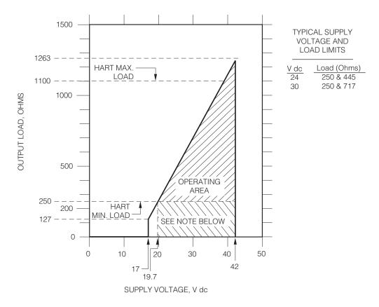
Figure 8. Supply Power and Loop Load
