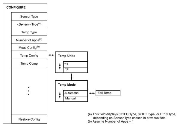
Figure 11. Example of Temp Config Menu Structure Diagram
