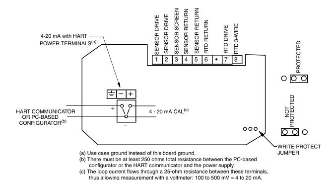
Figure 1. Wiring Connections for 876EC Transmitter
