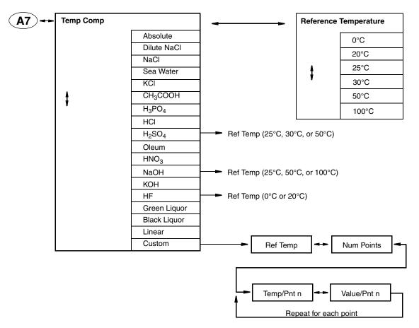
Figure C-7. Temperature Compensation Structure
