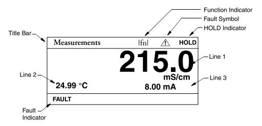
Figure 2. Sample 3-Line Measurement Display
