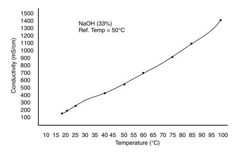
Figure 20. Configured Conductivity vs. Temperature Data
