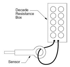
Figure A-1. Connection of Resistance Using Loop of Wire and Decade Resistance Box
