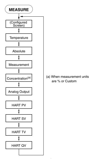
Figure 12. Measure Mode Structure Diagram
