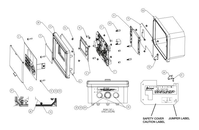
Figure 26. Exploded View of 876EC Transmitter
