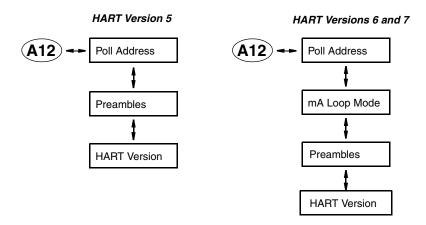
Figure C-12. HART Digital Structure
