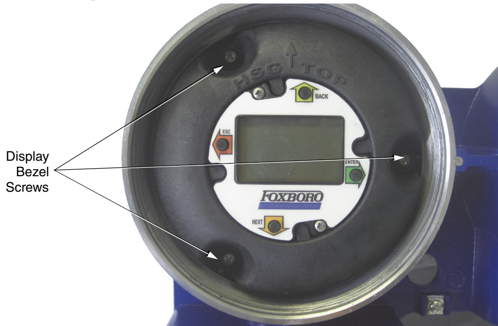
Figure 52. Loosening the Display Bezel Screws
