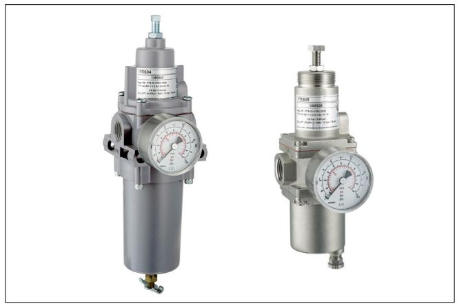
Control of instrument supply air pressure, and removal by filtration of dust particles and water content, to drive pneumatic actuators. FRS04 and FRS05 are dedicated for direct mounting to valve positioners SRD998 with pneumatic performance "High Air Output".
