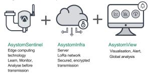
The **AsystomSentine**l beacon is a smart, connected, autonomous device capable of managing numerous integrated sensors (sound, vibration, **ultrasound**, shock, ambient and contact temperature, ambient humidity). The outdoor version also offers the possibility of connecting external sensors: 4 -20 mA, Thermocouple, Dry contact, PT 100.
